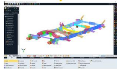
Design Enablers like bulk heads and beads from MeshWorks for Chassis Frame to aid what if studies and optimization
