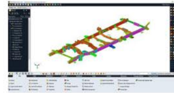
Import CAD and Create Mesh in MeshWorks
