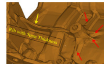
Rib creation using MeshWorks
