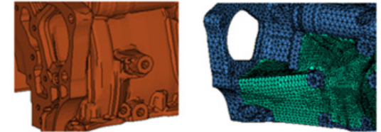
Rib de-featuring and design space creation using MeshWorks
